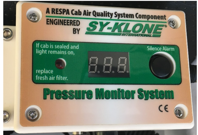
Cab Pressurizer Monitor. Alerts when Cab is not Pressurized.
